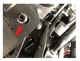
Once the 2 lower bolts are removed proceed to removing the hood & front end cover.
