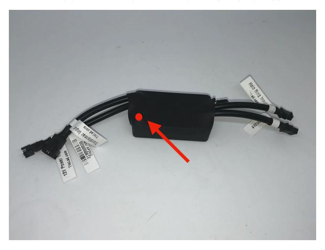
To program a new chaser remote, locate the small black push button on the module.
