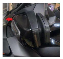
2. Remove the following screw with a torx 20 driver and slide actual mirror out of its housing. Be careful when removing screw, actual mirror is loose, do not drop the mirror.
