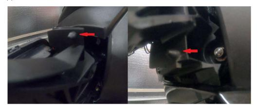
10. The last step is to put the cover back on the front of the mirror housing by sliding it back into its clips.
