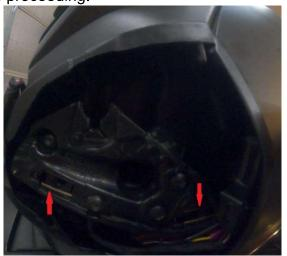
8. Return housing to bike and plug the electrical wire back in. Position the hanger bolt into its pocket and adjust mirror so that the bottom nipples can click back into its clips. You will hear the nipples click into place into the clips. Verify there is no play in the mirror. If so, remove housing and adjust the collar nut and jam nut to achieve no play in mirror housing.
