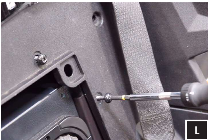
L. Replace the factory T40 torx screws to secure sub enclosure.
