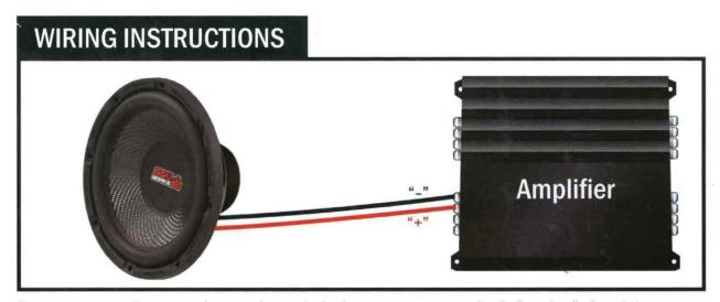
For proper sound, ensure the speaker polarity is correct connect the "+" to the "+" and the "-" to the "-"from the speaker wire to the amplifier. If using with an SSV Works complete system refer to the amplifier wiring instructions for more detailed wiring information.
