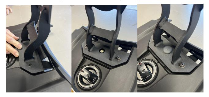
4.- Once the back rest frame mount is in place take the back rest and secure it to the frame mount with the 3 Phillips Screws and plastic cap covers. Once all screws are in place, you can adjust the height of the back rest once installed on your Spyder RT
