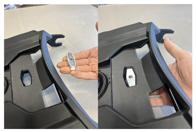
2.- Next take the base mount plate and secure it to the LinQ mount. The plate secures to the Linq with the two hooks that loop under the bar in the LinQ mount. Once in place take the Socket head bolt and washer and secure the base plate to the LinQ mount. Tighten down the bolt.
