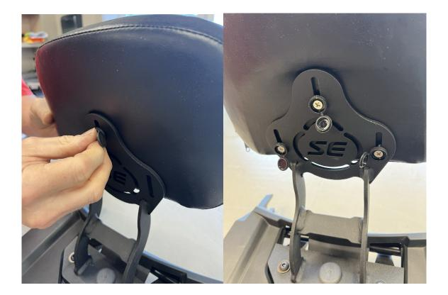
The backrest is now installed. Now you can take the whole unit and snap it into the rear to the Spyder. Be sure to lock the Linq mount in place.
