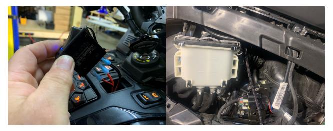
6.- Next remove the front panel shown below. Keep the two screws. Locate the factory accessory wire and keep it out in the open. Remove the plastic panel from the oem connector.
