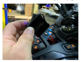
11.- The Light Bar wires plug into the ground wire on the switch and the open terminal as shown below. Then install the switch. Before reinstalling all panels make sure the light is working. You should be able to turn on the key switch and then test the Light Bar for final adjustments. Be sure to tie up all lose wire cables with the supplied wire ties.
