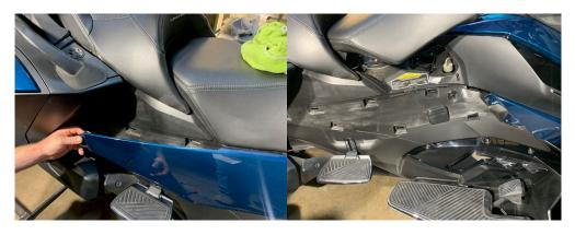
2.-Raise the seat to allow easier access to the docking station wiring. Next remove the upper blue panel shown below. Remove the 3 Torx screws shown. Then remove the 3 push pins under the front trunk.
