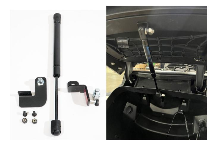
1.- First remove the center screw using a T-20 Torx wrench. Next take the upper mounting bracket. Remove the 3M tape back. Place the bracket in the center screw hole location and press the back of the bracket to the trunk lid to hold it in place. Next take the suppled new T-20 Screw that will recess into the bracket and tighten down. Then take the supplied ball mount and using ½: wrenches secure the ball to the mount as shown below.
