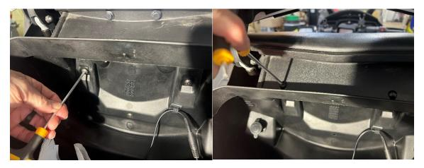
3.-Take the supplied template and place it in the space as shown below. It's designed to align perfectly. Then take a 7/32 drill bit and drill two holes through the template for the lower bracket mount.
