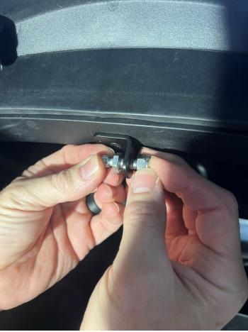
2.- Next remove the passenger back rest by removing the 3, T-25 screws suing the T-25 Torx wrench in the trunk. Then using the T-20 Torx wrench loosen the T-20 screws on the back seat panel as shown. Once those screw are loosened then remove the rear passenger backrest.
