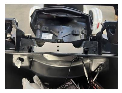
4.- Once the two holes are drilled, take the lower mount and the two supplied black T-20 screws and locknuts, and secure it to the trunk housing as shown. Use a 10mm wrench on the two lower locknuts to tighten them down. Finally take the gas spring with the larger receiver section of the spring at top, snap the spring on the upper ball and the same for the lower ball. Your Trunk lift kit is now installed.
