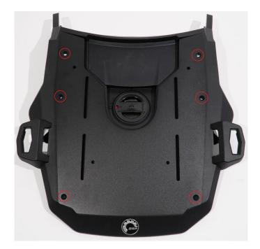
2.- Once the 6 holes are drilled take the suppled bolts, place a bolt in each hole with a spacer separating the plate from the rack. Then take a washer and locknut on each bolt and tighten down not to overtighten. Your Mounting plate is now installed.
