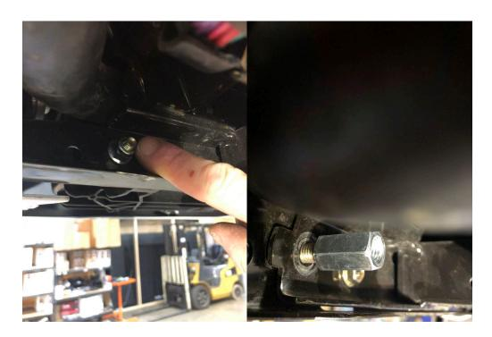
3.- Before installing your bumper, in reverse reinstall the plastic lower panels, screws, and push pins.
