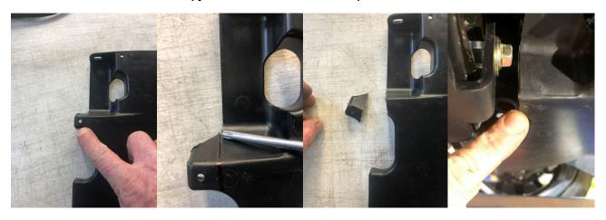
6.- Do the same for the left-hand lower panel as shown below. Trim the corner a shown, remove the piece and install.
