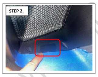
The (4) magnetic brackets provided in your kit will be attached to the inner fairing, depicted in red box in **STEP 2.** Pictures, with the 3M tape that is pre-installed on the brackets.
