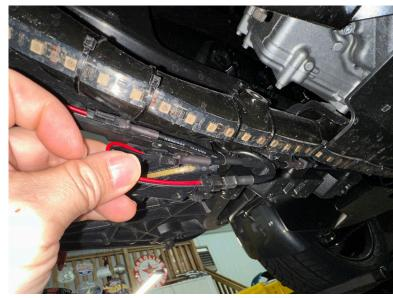
Locate the front floorboard LED and disconnect it from the extension. Apply di-electric grease to the 1:2 splitter (provided in the kit) and insert extension to the front LED and rear extension. Then re-connect the front extension to the end of the splitter. The front floorboard LED is the source of power to the rear boards.
