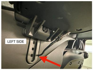
Pull out the panel slightly to insert the extension on the hole that was widened, with wire facing towards the rear of the Spyder. After the wire is inserted and snug, reattach the floorboard, then insert then tighten the original bolt back into the same hole position as before.
