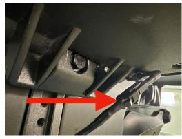
Use di-electric grease and connect the 24" extension to the LED.
