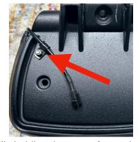
While holding the screw from other side, insert the cable tie, insert wire from LED, secure and place the locknut on the screw like shown above.
