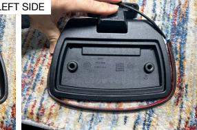
up. Position the LED around the lower perimeter of the boards with wire connector out towards the rear of the Spyder.
