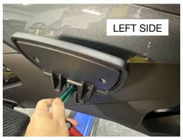
Lift up the passenger rear floorboard to reveal the bolt that holds the floorboard in place.
