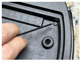
Insert 1 of the 4mm screws from the top of the rear hole of the floorboards.
