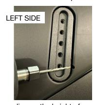
Depending on the height of your floorboards, you'll need to adjust where to drill to widen the slot for the wire to be inserted to the back of the panel. Do not pinch wire. Position the wire just under the boards, insert through panel and out towards the rear of the Spyder.
