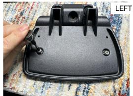
Flip over the board to remove the 2 allen bolts from the bottom that hold the rubber pad on the top side.
