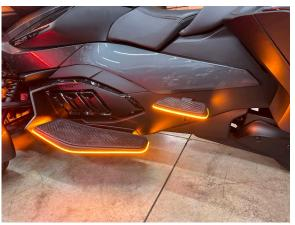
When all the connections are done, turn key to the on position and test for white running Led and turn signal functionality. Repeat installation process for the other side.
