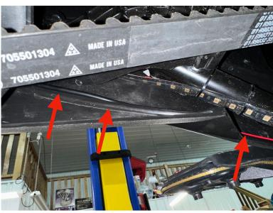
Run wire through the side plastic panel and zip tie towards the front. Make sure it is snug and not close to the belt.
