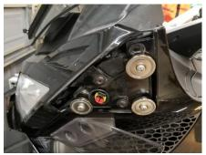
7. Install mirror: Secure the mirror with the new metal plates by hand and reconnect the electrical (secure electrical wires by dressing them back into the slot), then with CAUTION (magnets are powerful and will connect quickly) - line up the two bottom holes with the hex key bolt and gently guide the mirror onto the bike.
