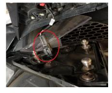
2. Once mirror is removed. Remove all 6 screws that hold the factory plates on.
