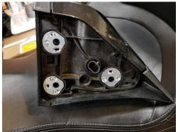
4. Bike: Remove the factory bolts from the bike using a 13mm deep well socket and remove the top T30 torx bolt. The T30 torx bolt will not be reused in the process. Discard or save the T30 torx bolt. Best Practice: Save T30 torx bolt, part can be used in other areas of the bike, if ever needed.
