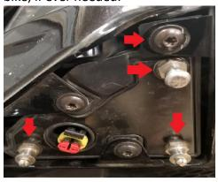
5. Remove 3 magnets, 3 bolts and 3 washers from the package. CAUTION, the magnets are powerful. The orientation will be: bolt, magnet, and washer (3 sets). Discard large washer separating the magnets. The large washers are only for shipping.
