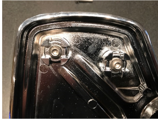
Bottom View of Left Floor Board w/ bolts installed
