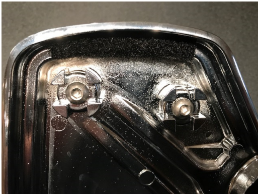
Bottom View of Left Floor Board, install Velcro on upper ledge as shown
