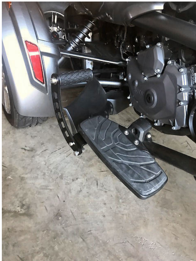
Left Side F3-T Road Peg Assembled on Floor Board
