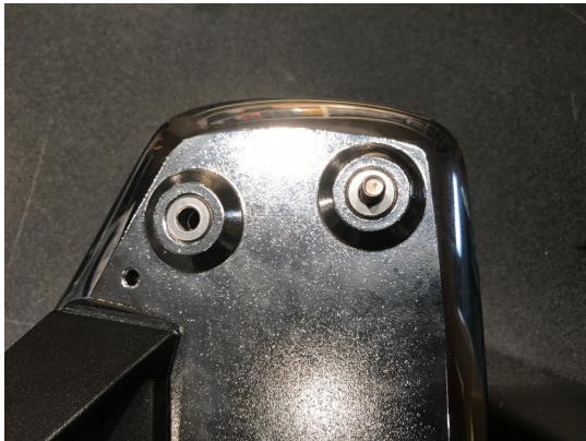
Bottom View of Left Floor Board, spacers & install bolts as shown
