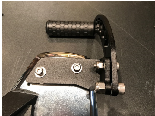
Bottom View of Left Floor Board Extension Installed tighten all lock nuts securely
