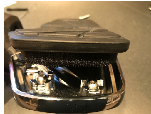
Bottom View of Left Floor Board Rubber Pad, install Velcro on upper ledge as shown Velcro will secure Rubber Pad to metal frame but allow access if needed
