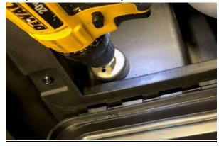
Remove the bolts for the lower driver side trim panel and the plastic clip under the drivers left arm guard located between the integrated roll cage and the body. Pull the lower side panel back, but there is no need to remove it completely, just enough to allow access to the side of the inner storage compartment so-as the bolts for the air tank mounting base can be installed.
