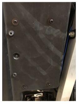
Install the bands and orient the tank so the mounting bases are directly opposite of the side ports on the tank. Position the tank in the compartment on the RIGHT and as forward to the opening as possible, allowing room for access to the drain plug. Mark the holes and drill where necessary. 2 bolts will be visible from the outside; however we have included black oxide button head bolts to retain an OE type look from the outside. Install the tank using those 4 bolts with blue thread lock on them.
