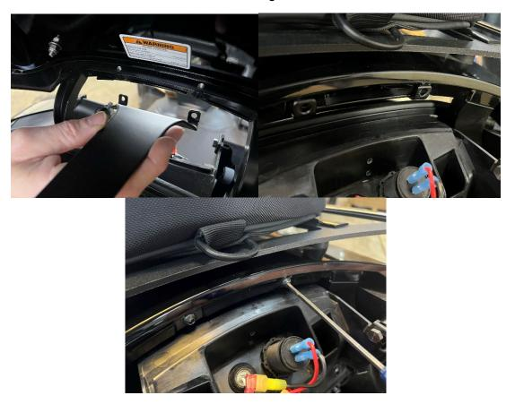
6.-Once the upper lift mount bracket is installed open the trunk, take the gas spring and snap each spring head socket over the 10mm stud bolt in each lift kit bracket. They are simple to push on.
