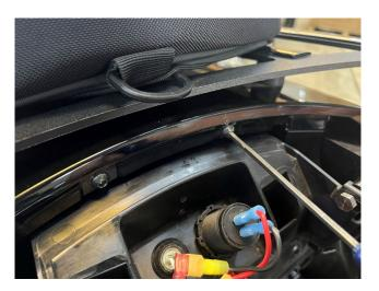
5.- Next take the upper lift kit mount and insert it from the trunk area so the mount tabs align with the two holes from the screws you just removed. Then take the 2 new supplied 6mm black screws and secure the mount to the trunk housing.
