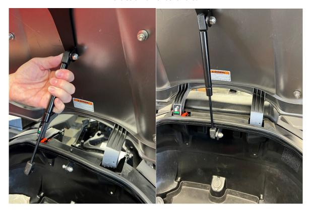
7.-You may need to adjust the trunk lid alignment stubs once the lift kit is installed. Remove the two push pins that hold on the cover as shown below.
