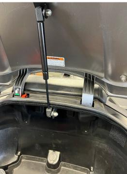
1.- First remove the two Button Head Black Screws that are used to hold on the rear Passenger Back Rest using a T20 Torx wrench as shown below. Then remove the rear passenger backrest.
