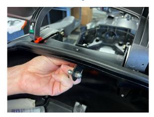
4.-Take the trunk lid and tilt forward to the front of the Spyder so it's easier to work on. Using the supplied template drill each side a 7/32" hole. Simply turn the template over to drill the opposite side.
