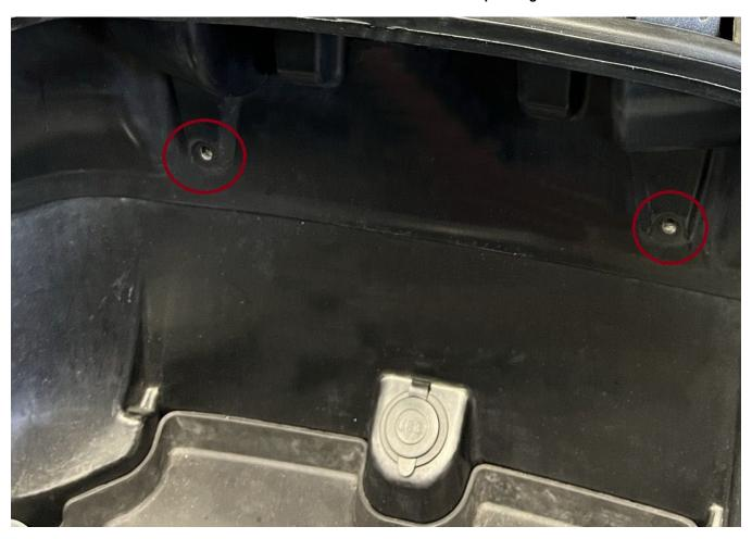
2.- Take the supplied template and place it as shown centered on the backrest mount. Hold firmly in place and drill two 7/32" holes.
