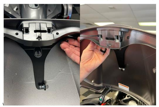
6.- Finally take the gas spring with the larger receiver section of the spring at top, snap the spring on the upper ball and the same for the lower ball. Your Trunk lift kit is now installed. Last reinstall the passenger backrest pad in reverse of how it was removed.
