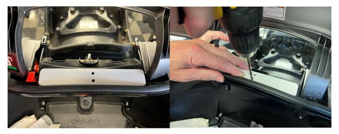
3.-Next take the supplied T-20 Screws and Locknuts and secure the upper mount bracket as shown below. Tighten down both nuts using a 10mm wrench.
