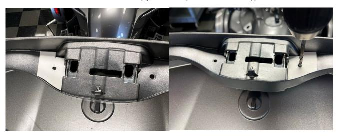
5.-Next take the upper bracket and locate it on the trunk lid as shown below. Take the two supplied T-20 Screws and Locknuts and screw the mount in place. The screw goes in from the top with the locknut on the bottom. Tighten down with a 10mm wrench. To simply the installation of the bracket you may lift the lid vertically.
