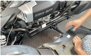
4. There are 3 positioning points on the removed side guards. Use a 5.5mm drill to drill out screw holes, then install the foot side guard
