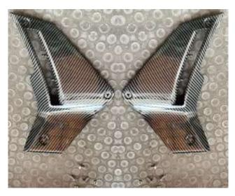
3. First remove the original vehicle cover, loosen the screws on both sides of the front bumper (without taking off the front bumper), remove the nylon snap fasteners that hold the side guards, and take off the side guards.
