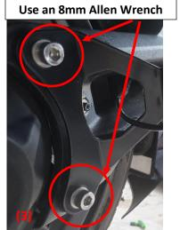
(1) Make sure that the upper rear brake caliper mounting bracket hole is aligned with the final drive unit upper mounting hole.
