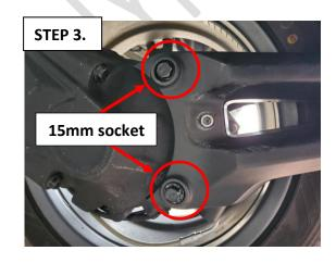
While holding onto the rear of the fender to relieve tension on the top bolt, remove only the top rear brake caliper retaining bolt using a 15mm socket wrench and allow the lower the fender support bracket to slowly pivot on the bottom brake caliper bolt until it is sitting on the ground.
