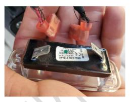
**STEP 1.** Begin by using a T25 torx screwdriver to remove the 2 torx screws from the license plate LED located under the front lip of the rear fender trim cover then remove the T30 torx screw.
