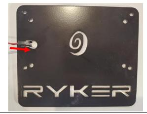
Next you will route the 2-pin female connector from the end of the wires coming off of the LED USA flag and route it through the hole in the RYKER mounting plate.
