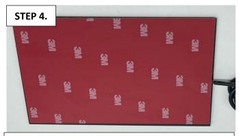
Before peeling off the red 3M plastic from the back of the LED USA flag, make sure the surface of the mounting plate is cleaned & prepped with the alcohol & adhesive pads provided. Wipe the surface of the plate with the alcohol pad, let the alcohol dry, then wipe the area with the adhesive promoter pad and let dry.
