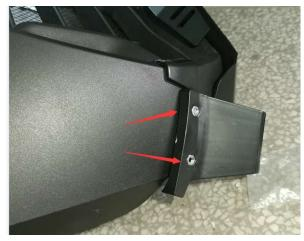
4. Clamp the narrow section of the air inlet onto the mounting bracket, and attach the wide end to the upper part of the middle net on both sides, and drill with a 5.5mm drill bit.
