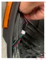
Wrap the connectors with electrical tape to protect it
