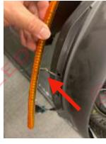
Position the new yellow LED over the mounting position and mark for the wire hole to be drilled. Drill large enough for connector to pass through. Clean surface with alcohol supplied, let dry. Apply the primer tube to the area and let dry. Peel off backing and adhere LED to the fender and press firmly. Be sure to warm up the adhesive if your installing in temperature cooler that 70 degrees for maximum adhesion
