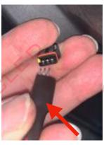
Slide the shrink tube thru the wire harness supplied with the pins exposed
