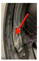
Gently tuck in the wires under the front tip light pocket
