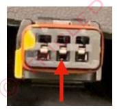
APPLY DI ELECTRIC GREASE TO ALL CONNECTIONS Insert the supplied pin harness into the factory harness. Note the slots where the pins are inserted has metal pin.
