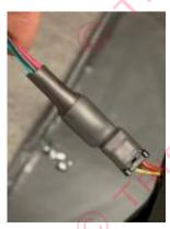
Slide the shrink tube over the pins and into the Oem connector as far as it will go up. Use heat gun or lighter to shrink the tube tightly, let it sit for a few minutes to cool and hardens
