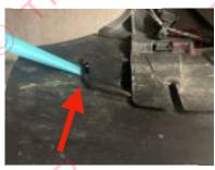
Use a pry tool to release the small tab from the bottom front fender that holds the tip LED
