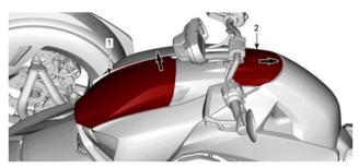
3. On the left side of vehicle, remove and keep the four (4) plastic rivets.
