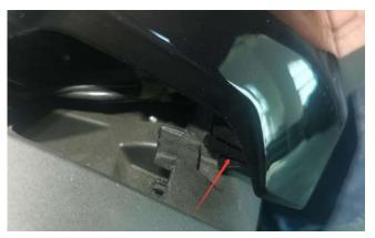
3. Push the hood in the direction of the arrow to install it.
