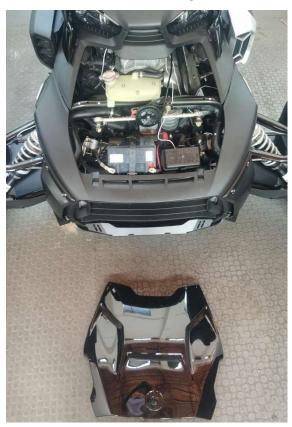
2. Align the clip on the hood with the mounting hole on the vehicle body.
