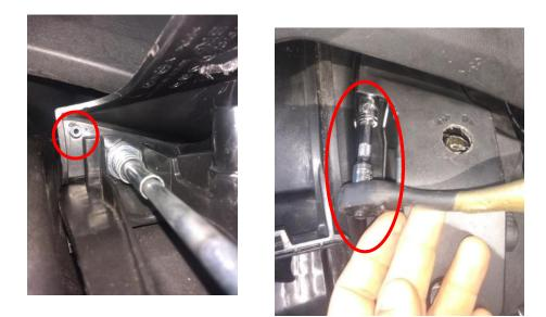
While holding down the barrel adjuster, place the washer over the adjuster then start threading the 10mm nut that was removed in STEP 11 onto the bottom of the adjuster. Use a 1/4" 10mm deep socket
