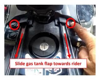
Remove the upper-fairing by sliding the fuel tank flap towards the rider. Assembly open and removing the pushpins.
