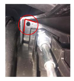
Insure that the 1/4" drill bit is centered along the top left corner of the parking brake lever housing as in the picture circled in red before you drill the hole.
