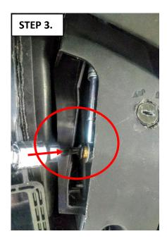
Use a T30 torx bit to remove the side M6 X 16 torx head screw from the parking brake lever cable connection point.
