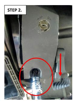
**Ensure that the park lever is disengaged** which should be pointed towards the ground. Use a T30 torx bit to remove the bottom M6 X 16 torx head screw.
