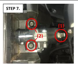
(1) Disconnect the positive and negative ports from the back of the glove box USB connector.
