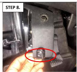
Pull lightly on the bottom of the parking brake lid to expose the top left corner where you will be drilling a hole with a 6mm drill bit for top mounted barrel adjuster.
