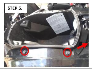
Remove side-fairings by removing 3 pushpins from both sides.
