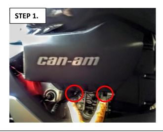
Release the 2 cover retainers from the bottom of the air filter service cover located on the left of the RYKER by the parking brake, lift up & away from the RYKER. This will expose the park lever mechanism.
