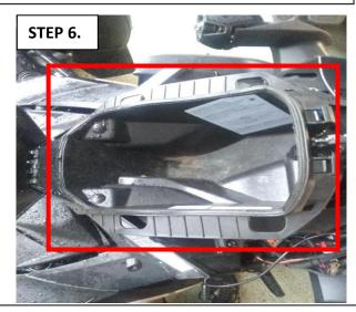
Before removing storage compartment (FRUNK), disconnect the USB connector.
