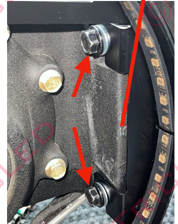
Loosen these two swing-arm attachment bolt, just a few turns to allow the new wheel rings to slide over the two bolts.
