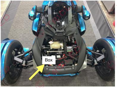
You will be making connections to the original module box. Use one of the open ports for kit #3
