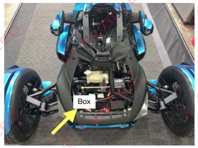
You will be making connections to the original module box. Use one of the open ports for kit #2
