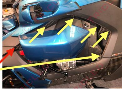
Repeat for right side Connect the 36" extension to the left LED strip and route the wires to the right side(throttle side). Connect 1:2 splitter to right side LED and connect the left side extension to the 1:2 splitter.
