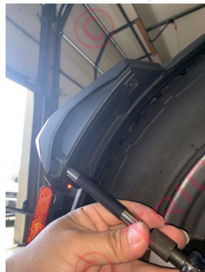
Remove screw with torx 20 bit
