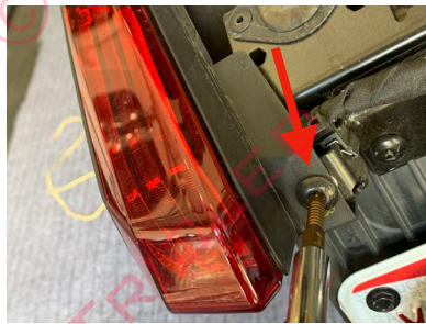
Remove taillight bolt using Torx 30 bit
