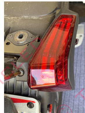
Remove taillight bolt on using Torx 30 bit
