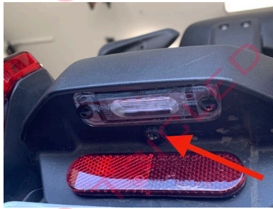
Remove screw with torx 20 bit
