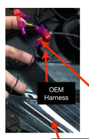
With the back lid open locate the factory harness that plugs into the left (driver) rear tail-light. Pull the harness up to reveal wires. Peel back the OEM wire insulation. Install and crimp the 3 supplied T-tap on the (green/pink stripe), (White/Pink) and (black) wires.
