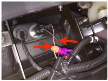
3. To power the LED's, connect and join both sides together (Positive + black/wht stripe)together and separately (negative black) together with the other side. You will need an extension from one side to reach the other side Depending on how your connecting. If you are not using a fusebox you can connect both positive and negative wire to the cigarette plug harness located just in front of the passenger firewall.
