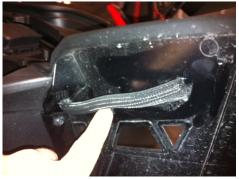
2. Loom the wire and resistor and use one of the mounting square to adhere to the back of the fender as support. Clean the surface for reflector mount and also for the backside. Do this for both sides at the same time to get maximum use out of your primer. Do not pull wire from resistor box as this piece is fragile and controls the entire lighting. Mishandling is not covered under warranty. Zip tie wire with resistor and loom to the square tab.
