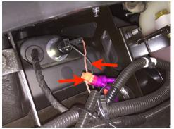
3. To power the LED's, connect and join both sides; Positive wires together and negative wires together. (+ is Black/white stripe)(- is solid black) You will need an extension from one side to reach the other side, depending on how you are connecting them. If you are not using a fusebox, connect both positive and negative wires to the cigarette harness located just in front of the passenger firewall.
