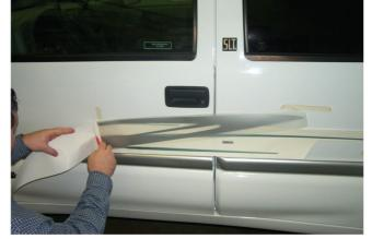
4. Temporarily secure the end of the graphic to the vehicle surface and cut the backing paper off near the center hinge.
