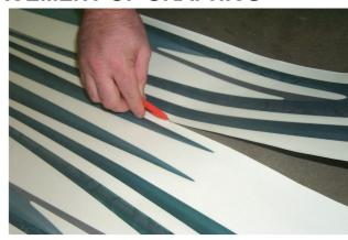
1. Using your Snappy knife, carefully cut the component graphics apart from each sheet, if needed.
