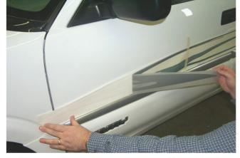
3. Remove the positioning tape on either side of the center hinge from the first panel and peel the liner paper away from this portion of the graphic. Lightly tape the graphic to the vehicle surface (as illustrated in Step 4).
