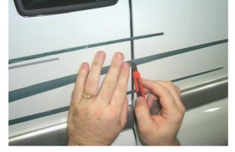
9. Trim away excess graphic material from door edges by inserting the knife along the edge of the opening at a 45-degree angle. Then carefully cut through the vinyl on both sides of the seam and remove the scrap.
