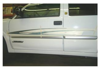
2. Tape the component graphic panels onto the side of vehicle to determine exactly where you want the graphic panels installed. Apply a strip of tape vertically through the center of each component and lightly tape each end of the graphic panel to the vehicle.
