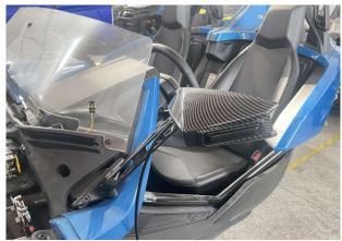
3. Pull out the harness on the turn light of the original vehicle and connect it with the adapter wire configured for the side view mirror cover trim. Place the harness of the side view mirror cover trim along the vehicle harness to the place of the turn light (the harness can be fixed with ties), and then connect it with the adapter wire. (Install the other side mirror cover trim according to the same procedure).
