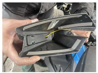
2. Clip the side view mirror cover trim onto the side view mirror and press hard to make it fit better with the side view mirror.
