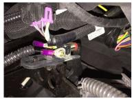
Once the new manual switch is mounted, be sure to tighten down the 10mm bolt and have someone push the brake pedal again to ensure contact when the brake is pressed down to engage the switch. Make fine adjustment to ensure it makes contact and the rear brake light is working properly. When the brake pedal hits the red switch the brake lights are activated.
