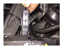
Locate the wire that is attached to the magnetic switch and disconnect it from the factory harness. You will connect the new brake switch to this same OEM connector.
