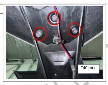
**STEP 1.** Begin by removing the OEM license plate bracket by using a T40 torx screwdriver to remove the (3) T40 torx screws located under the rear deck.
