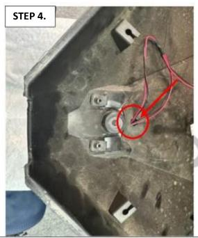
**STEP 4.** Feed the 2 remaining connectors thru the small hole of the bottom panel. One male 2 pin connector is for the new SLINGSHOT plate LED and the other 2 pin male connector for the OEM license plate LED.
