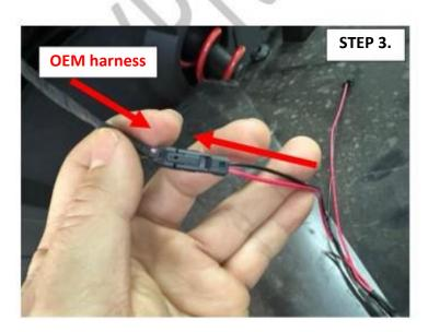
**STEP 3.** Your kit will come with 2 harnesses. A main 1:2 harness that connects to the OEM harness male connector to the OEM small license plate light. The small harness is provided to accommodate all Slingshot from 2015-current models. The wiring may be reverse on certain years and models.
