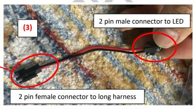
**STEP 6.** Add some die-electric grease to the connectors before you connect the **(1)** female connector from the SLINGSHOT LED plate to the **(2)** male connector from the provided 1:2 harness. Once you have made the connection, turn the key on your Slingshot to test the LED to insure it activates before securing the harness with a zip tie as in the
