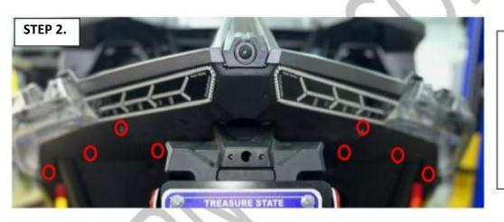
STEP 2, Use a T40 torx screwdriver to remove the (8) T40 screws holding the bottom panel on. Slowly lower the bottom panel so that you have access to the OEM harness and disconnect the OEM license plate LED.
