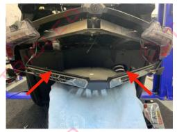
Remove the license plate bracket and Torx 40 bots that hold the lower plastic cover
