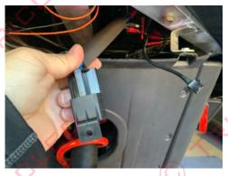
Remove the OEM harness from the left and right tail lights and connect the provided OEM harness inline and reconnect
