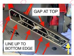
Position the new LED module on the surface, do not adhere yet!
