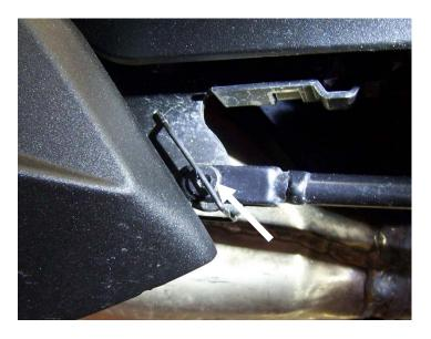
3. Remove two Button Head Screws (one on each side [front and rear]) that holds the Foot Peg on. Be careful when removing the Foot Peg as there are threaded brass inserts with two small ears that the Button Head Screws thread into. These ears line up with slots on the Foot Peg. They can be easily broken off!!
