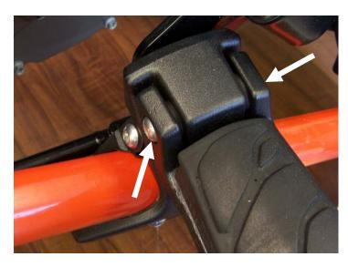
4. Loosen the two Button Head Screws (one on each side [front and rear] of the Outside, Slider).
