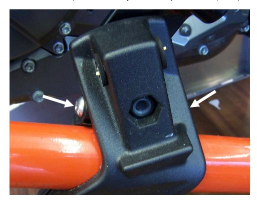
5. Remove two Button Head Screws that clamps the Outside, Slider and the Inside, Slider to the Footrest Support Tube. These two screws and the Nut Plate for them will not be used.
