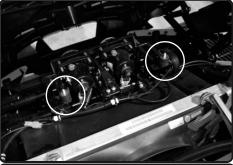
9. Secure and tighten the vibramounts.
