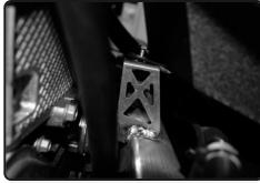
**11.** Now secure the back bracket to the factory air box mounting postion. Secure using provided m6 hex screw and fender washer.
