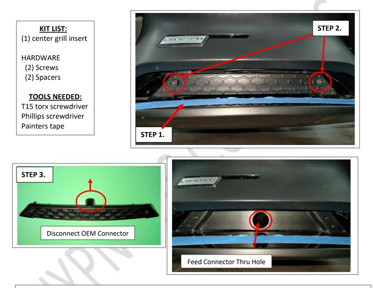
Before beginning the installation, ensure that the front of the fairing is clean and free of all dirt and oil.
