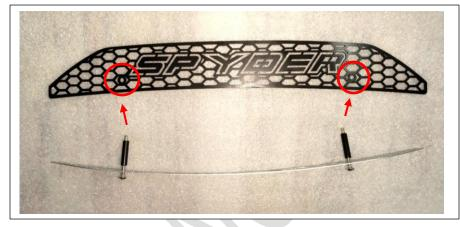
**STEP 4.** Before installing your new center grill insert, slightly flex the grill insert carefully so that it fits the contour of the mounting location.
