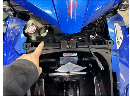
Open front trunk and remove service cover
