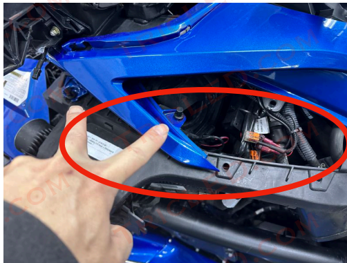
Remove top dash panel clip and exposed as shown in next step
