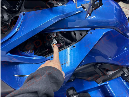
Remove top service panel cover from both sides
