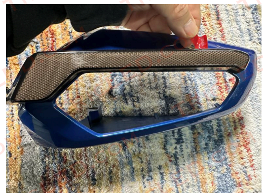
Position the new LED to the mirror cover. Note the cutout of the mirror is shaped to go around the bottom of the LED. Clean surface with alcohol.
