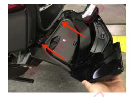
Drop the door down until the hinge comes off the pivot point and pull out towards the side. Working with the saddle bag off allows for better control while installing. Repeat for both sides.
