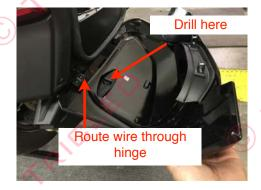
Remove factory triangle reflector. Using a heat gun or hair dryer is a good way to soften the adhesive for easy removal. Once removed position the new reflector and note where the center of the wire exits the back. Drill a hole through the case large enough for the quick connect
