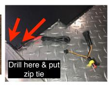
Drill a 3/16" hole on the back side of the bumpskid. This will hold the wire cleanly.
