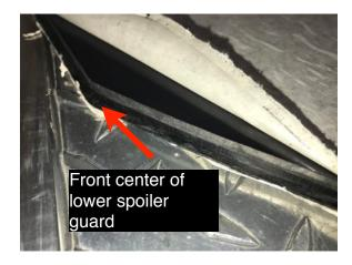
Position the LED on the lower lip of spoiler. This will serve as a base for the light to sit on. This lower lip helps guard the LED from accidental bump from underneath.
