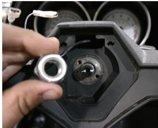
In some cases the steering wheel will pull off just using your hands. Most of the time though, a steering wheel puller is necessary. Steering wheel pullers are available online through several sources, including [Slingmods.com](http://Slingmods.com).
