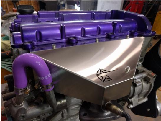
The DDMWorks Exhaust Heat Shield is designed to keep excess heat from your exhaust manifold out of your engine bay. This Stainless Steel Heat Shield also dresses up your engine compartment and makes things look much nicer.
