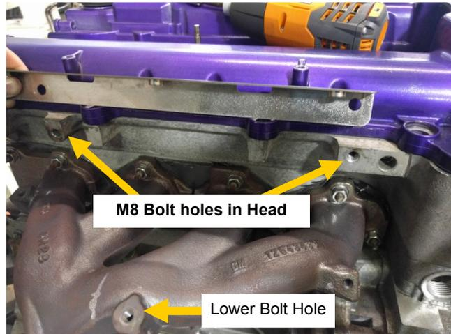
2. We will begin with the Heat Shield Bracket and the M8 Bolts with Washers. There are two threaded holes in the head of the engine that the heat shield will line up with. Using the M8 bolts supplied place one M8 washer over each bolt before putting the bolt through the Bracket and then into the holes in the Head of the engine. With both bolts in place you can tighten them down.
