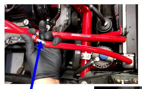
Join the line from the radiator to the line that goes up to the back of the coolant surge tank on the passenger side.
