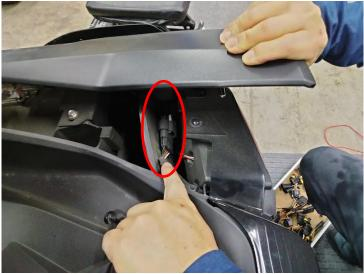
**STEP 8**. Disconnect the OEM taillight connector. Before connecting the new 5 pin connector that is provided in your kit, add some die -electric grease to each end. You will use the 2 pin male connector for the extension wire provided for the next step.
