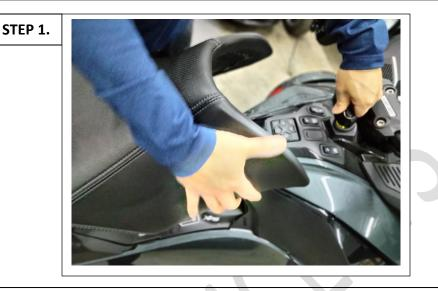
**STEP 1.** Remove the main seat by pushing the key into the ignition switch while turning the key counter-clockwise until the latch releases the seat.
