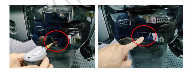
STEP 10. Remove the OEM antenna located on the left side above the cargo bin by turning the antenna counterclockwise.
