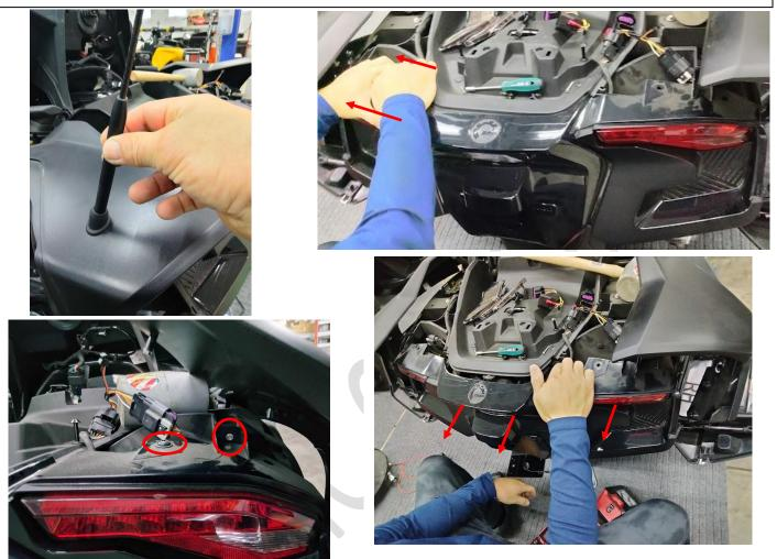
STEP 11. Next, take the wire extension provided in your kit, connect the female end to the 2 pin male connector on the new harness connector & route the male 2 pin connector end of the extension behind the taillight assembly down towards the backside of the license plate mount location where you drilled the 9/16" hole in STEP 9.
