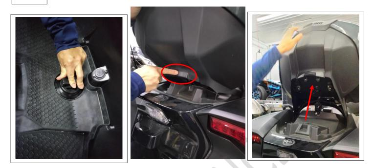
**STEP 4.** Open the rear trunk hatch and release the trunk lock be turning the center knob counter clockwise. Once the trunk lock is released, push the latch release on the back of the trunk that will allow you to tilt the trunk on its hinge.
