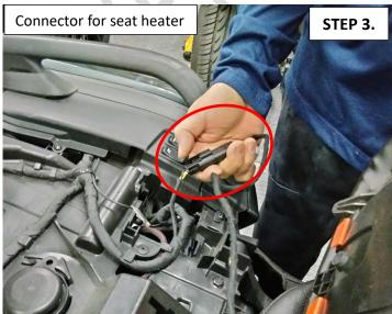
**STEP 3.** Before removing the passenger seat, you will need to remove the OEM seat heater connector.
