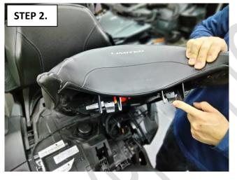
**STEP 2**, Remove the passenger seat by pressing the 2 tabs holding the front of the seat down.
