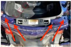
2. On the top rear trunk remove (4) bolts T30 Torx head.
