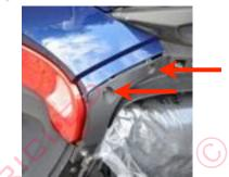
Start by opening both saddle bags and top rear trunk. Remove the two T30 Torx head screws on each side.
