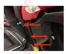
4 Remove shock from the top and remove the 2 bolts behind shock.
