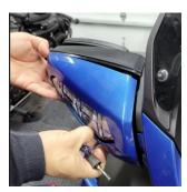
2. Remove the following screw with a torx 20 driver and slide actual mirror out of its housing. Be careful when removing screw, actual mirror is loose, do not drop the mirror.
