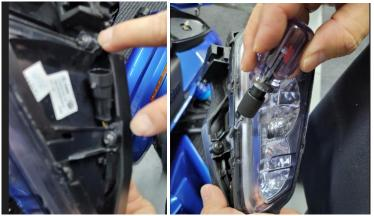
9. Remove the three bolts in the mirror housing.
