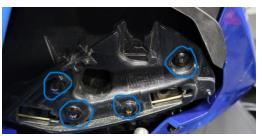
6. Take three of the bolts and place them in the holes as shown from the back to the front. After placing the bolts through the holes, put one nut for each bolt and tighten.
