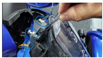
10. After the bolts are removed, line up the holes in the mirror housing with the bolts sticking out and then place the nuts and tighten all nuts.
