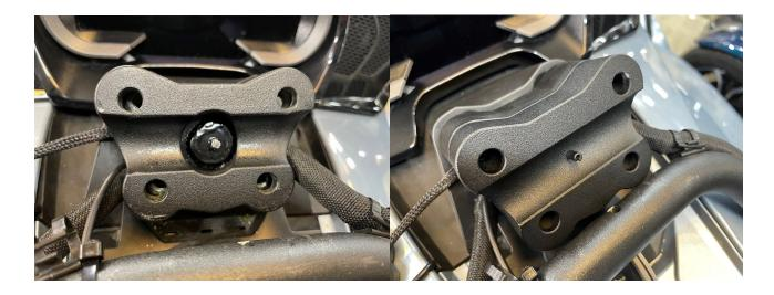
2.- Next take handlebars and relocate them as they were in the new cradle of the new riser, install the oem cap and use the new 4 socket head bolts. Use Blue Loctite on these 4 bolts and secure them in place making sure before you tighten them down securely that the handlebar position is correct. Sit on the Spyder and adjust the position of the handlebars to your comfort and then tighten down the top bolts snug then the bottom bolts then all four bolts evenly.
