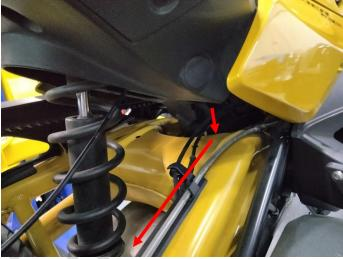
**STEP 4**. Route the extension wire along the OEM wiring and brake line that is secured to the swing arm.
