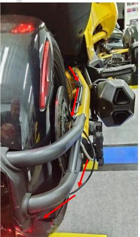
**STEP 5**. Before attaching your SPYDER plate to the F3, make sure that the wire leading from the LED is routed to the right of the mounting area depicted in the red arrow below.
