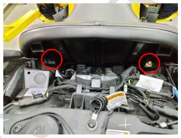
**STEP 2.** Disconnect the OEM rear taillight connector located on the right side of your F3 and connect the small harness provided in your kit. Before connecting the harness provided, add some die-electric grease to each end of the connectors.
