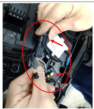
**STEP 3**. Take the extension wire provided in your kit and connect the 2-pin female end to the 2-pin male connector from the small harness that you connected to the OEM connector in **STEP 2**.
