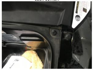
2.- Remove the access panel right above by pulling it off. This will give access to the battery.
